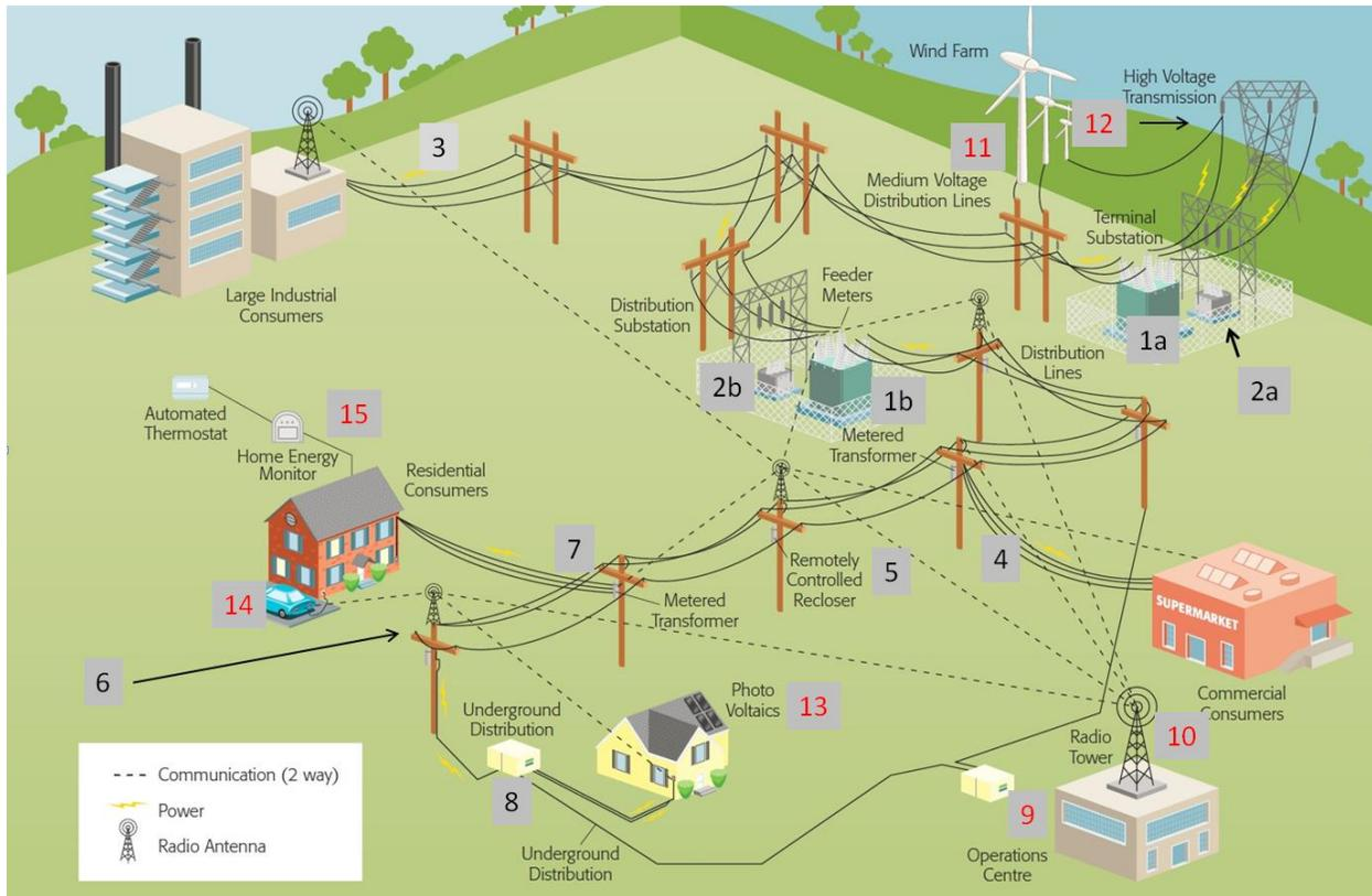
**Figure 3.2. Conceptual Schematic of 21st Century Utility Distribution System Topology<sup>69</sup>**
