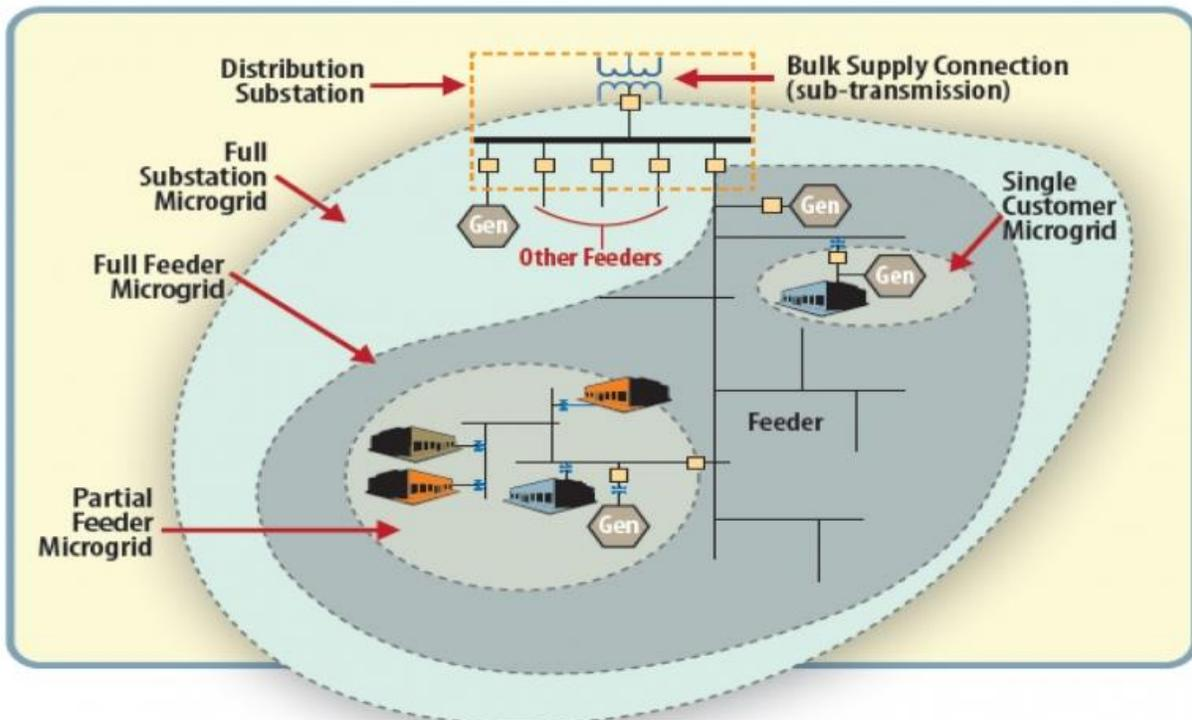
**Figure 3.13. Three Microgrid Schemes<sup>91</sup>**
