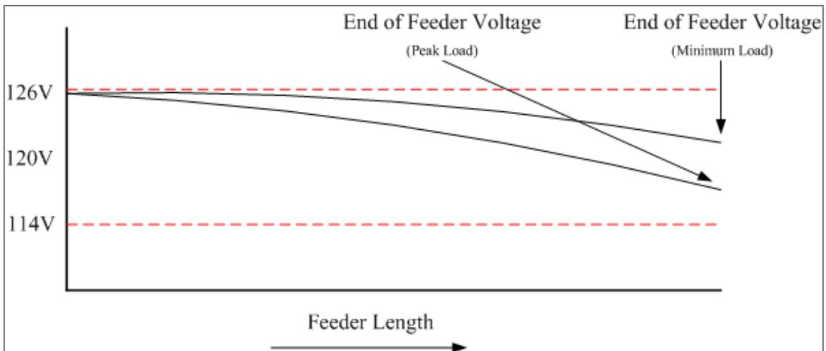
**Figure 2.17. Voltage Decrease Over the Length of a Distribution Feeder<sup>46</sup>**
