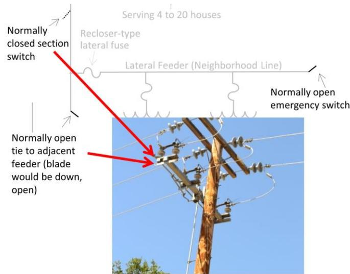
**Figure 2.16. Sectional Switches on Circuits Can Be Normally Open or Closed**
