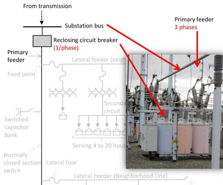
**Figure 2.11. A 12.47 kV Distribution Circuit where It Exits the Distribution Substation**
