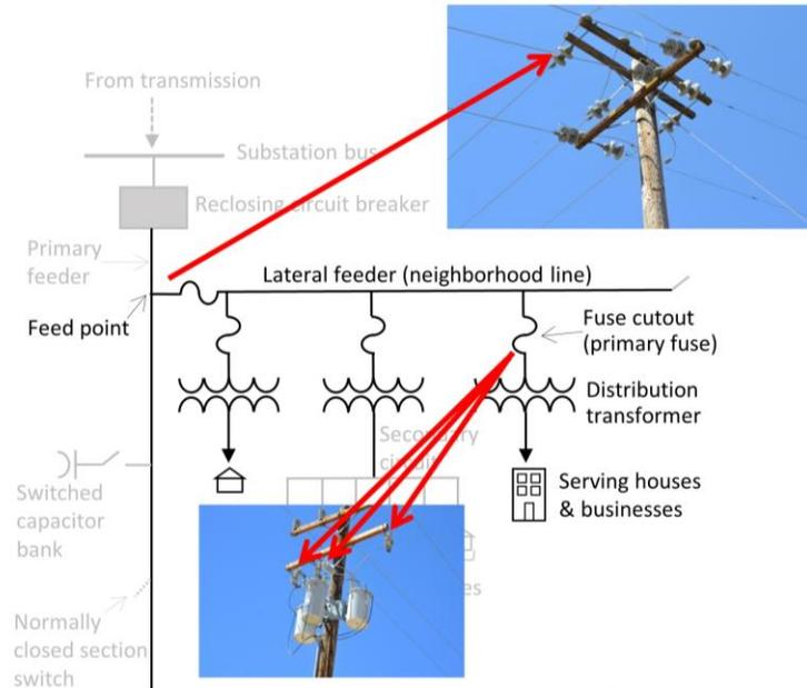
**Figure 2.12. Connection between Primary Distribution Circuit and Laterals Serving Customers**
