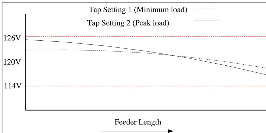
**Figure 2.18. Illustration of Two Regulator Tap Changer Settings to Manage Voltage Sag during Peak and Minimum Demand Periods<sup>47</sup>**
