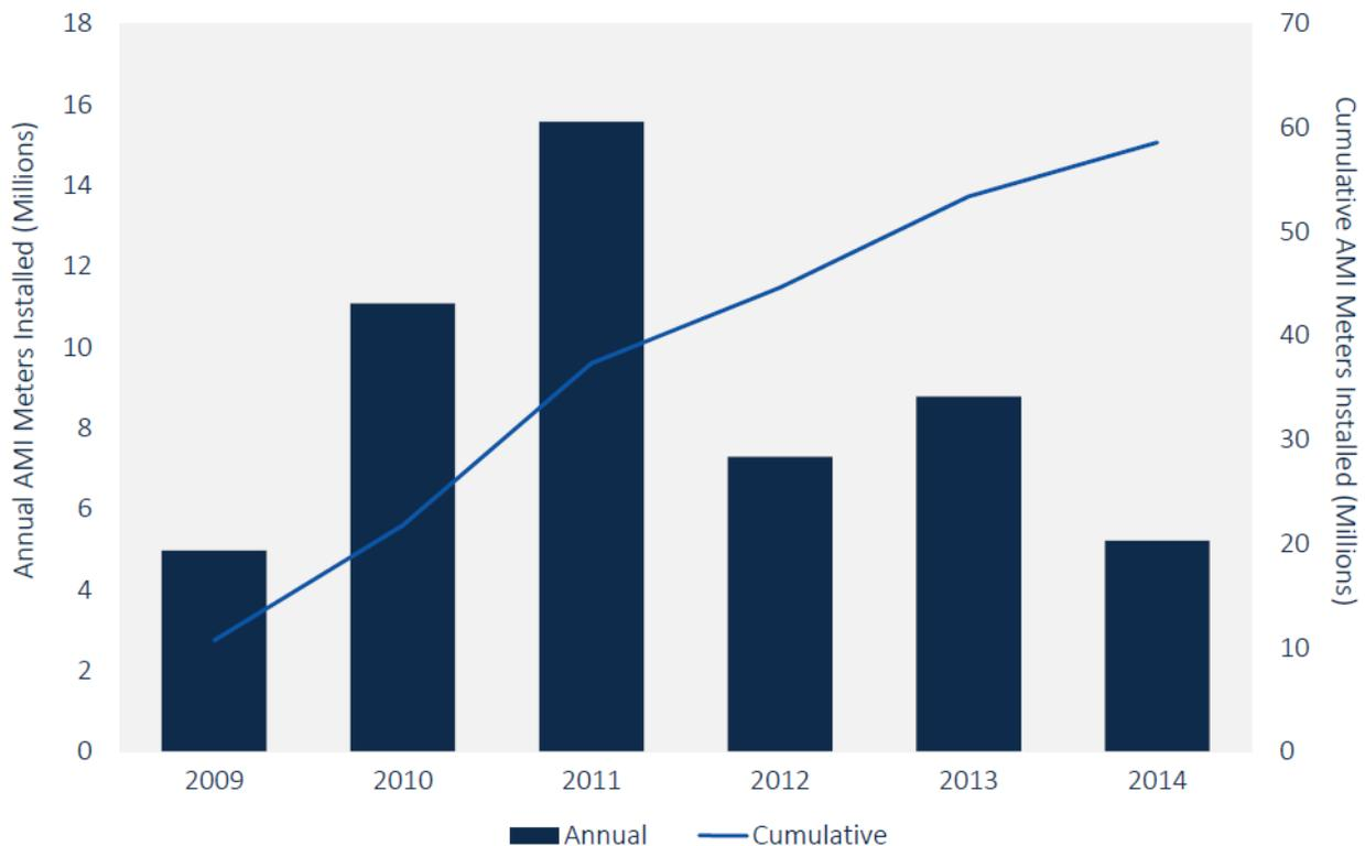
**Figure 3.8. Estimates of Advanced Meter Penetration in the United States<sup>81</sup>**
