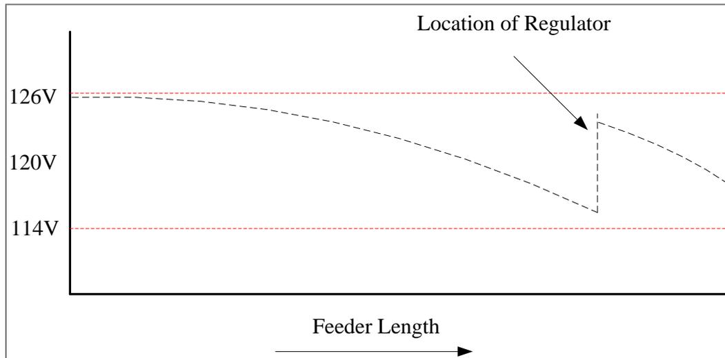
**Figure 2.19. Illustration of Voltage Regulation on a Feeder with Voltage Sag Outside of the Standard Range<sup>48</sup>**
