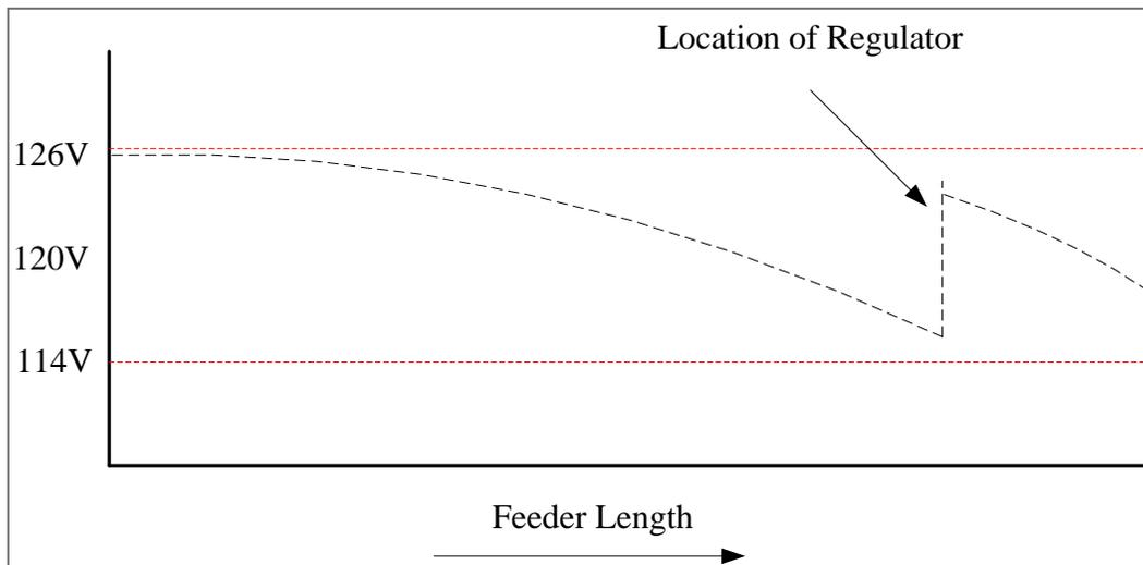
**Figure A.3. Voltage Regulation Using Supplemental Regulators<sup>19</sup>**
