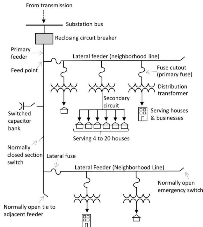
**Figure 2.10. Diagram of a Typical Feeder Construction<sup>44</sup>**
