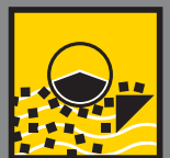
Wet Drum Separator
