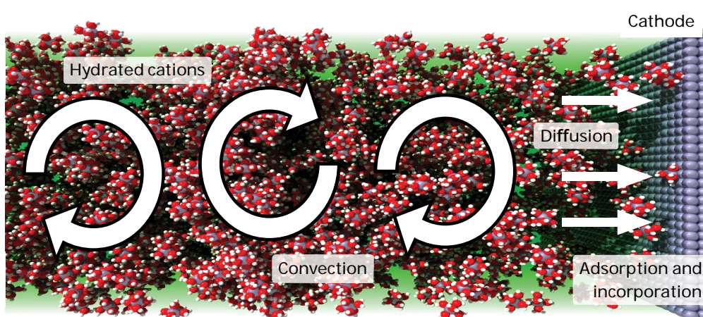
Fig. 135: Material transport from the electrolyte means i) transport by convection, ii) transport by diffusion, iii) hydration layer removal, and iv) adsorption onto the cathode.
