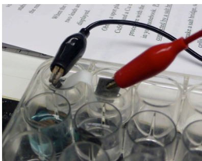
Figure 3. Electrochemical Cell Set Up
