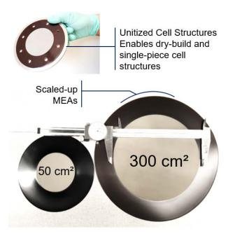
Figure 2. Membrane scale-up, unitization, and dry assembly
