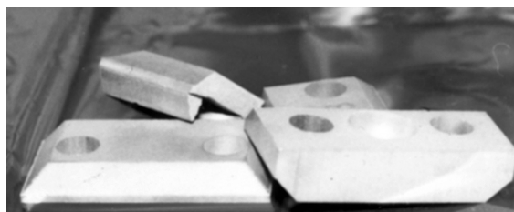
Fig.17. Component “plate”, 65 g, thickness 11.5 mm, density ~6.5 g/cm 3 [28].
