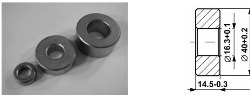
Fig.19. The rollers in size: 22, 30 and 40 mm diameter; G = 14 g for 22 mm, 105 g for 30 mm, 170 g for 40 mm and the dimensions in mm of a roller presented with tribological properties [28,34].
