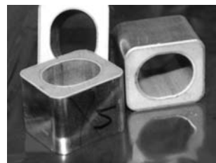
Fig.18. Component “cube”, 90 g, height 24 mm, density 7.0 ± 0.2 g/cm 3 [28].
