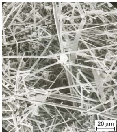
Fig.5. As in Fig.4 after treatment for 60 min at 1000°C in H 2 . SEM
