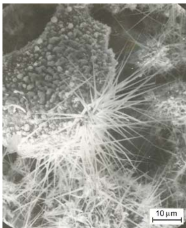
Fig.3. Surface of an electrolytic manganese plate annealed for 15 min at 900°C in hydrogen, oxal (alumina) boat. SEM.
