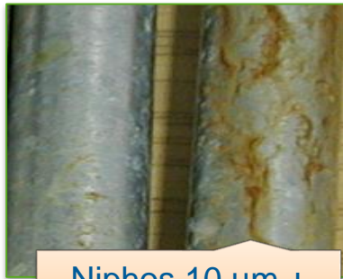
Niphos 10 µm + Cr 10 µm, 240 h
