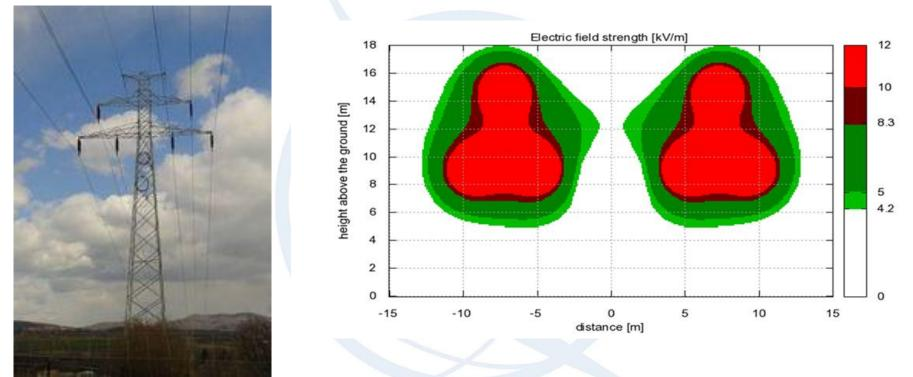
EMF in the vicinity of medium-voltage (MV) and high-voltage (HV) power lines at power frequencies (DC, 50 Hz, and 60 Hz); Software: **IFACDC** EMF & 5G implementation, F. Lewicki, 02.07.2020
