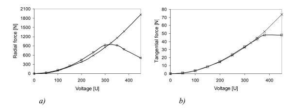
Figure 5.3. The amplitudes of a) the radial and b) tangential component of the force as a function of supply voltage at no load at 25 Hz whirling frequency for the 15 kW induction motor at no-load condition. Marking: x - linearized,  $\Box$  - normal.
