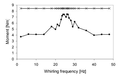
Figure 5.5. Moments in symmetric conical whirling motion with whirling radius 20  $\mu$ m. —•— measured and —X— calculated
