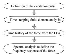
Figure 3.3. The flow chart of the force calculation by impulse method.
