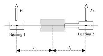
Figure 4.2. Axial rotor geometry of the test motor. ● centres of the bearing magnets ○ centres of the position sensors ↓ the forces acting on the magnetic bearings
