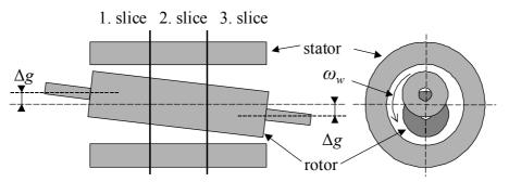
*Figure 3.2. Conical motion of the rotor modelled by multi-slice technique.*  $\Delta g$  *is the whirling radius.*
