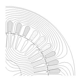
Figure 4.1. The Cross sectional geometry of the test motor.
