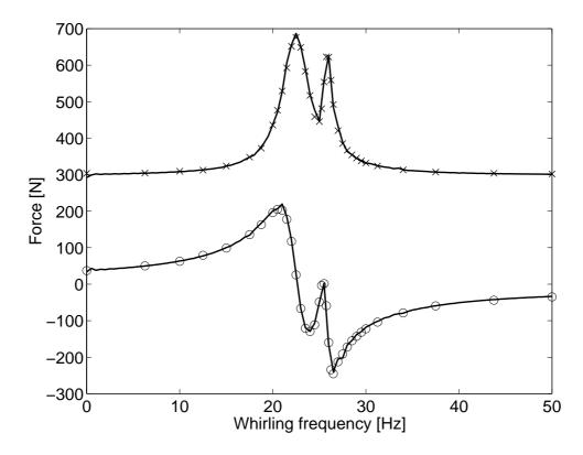
Figure 5.1. Electromagnetic forces calculated by a forced whirling and impulse method for a 15 kW induction motor at rated load (s = 3,2%). The results of the forced whirling method are marked by **x** for the radial and  $\circ$  for the tangential component. The continuous lines present the results of the impulse method.
