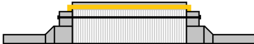
Figure 2.4 Laminated rotor with embedded squirrel cage [22].
