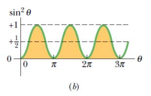
**Fig. 31-17** (a) A plot of sin  $\theta$  versus  $\theta$ . The average value over one cycle is zero. (b) A plot of sin<sup>2</sup>  $\theta$  versus  $\theta$ . The average value over one cycle is  $\frac{1}{2}$ .
