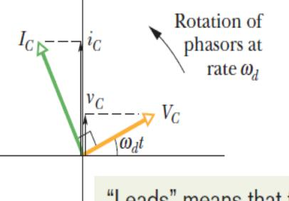
"Leads" means that the current peaks at an *earlier* time than the potential difference.  $\cos \omega_d t = \sin(\omega_d t + 90^\circ).$
