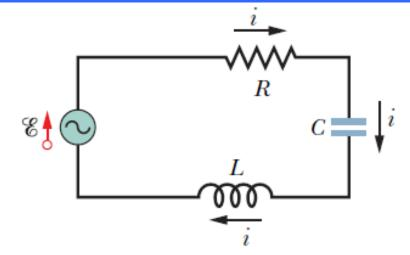
The natural angular frequency  $\omega_0$  is determined by the RLC circuit. The driving angular frequency  $\omega_d$  forces the oscillation to follow.
