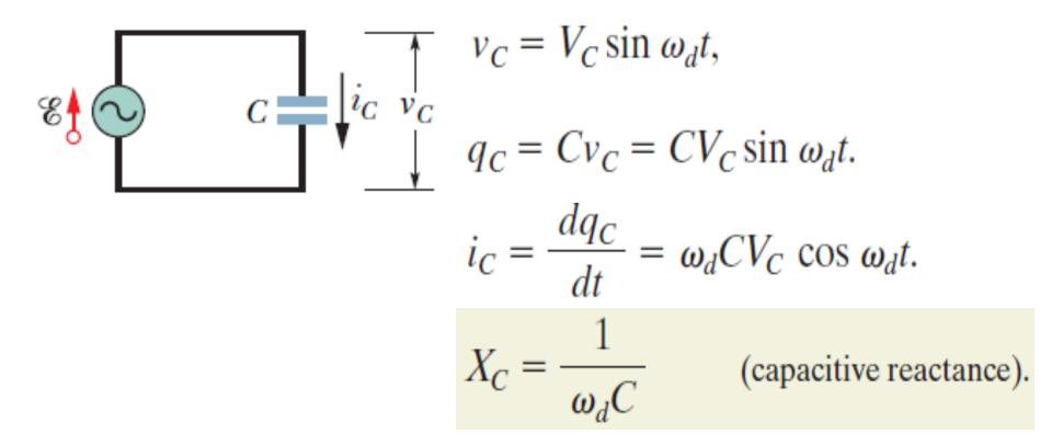
$X_C$  is called the **capacitive reactance of a capacitor.** The SI unit of  $X_C$  is the *ohm*, just as for resistance *R*. Exam R, C and L individually 2, only a capacitive load
