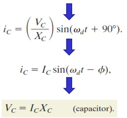
The current in the capacitor leads the voltage by  $90^{\circ}$  <sup>14</sup>
