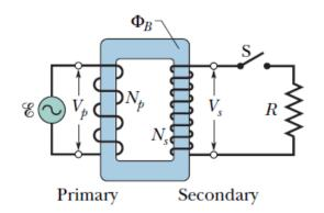
**Fig. 31-18** An ideal transformer (two coils wound on an iron core) in a basic transformer circuit. An ac generator produces current in the coil at the left (the *primary*). The coil at the right (the *secondary*) is connected to the resistive load *R* when switch S is closed.
