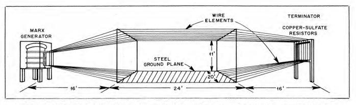
Fig 11—A drawing of the large parallel-plate EMP simulator used in the tests. The Marx generator is a high-voltage pulse generator in which several capacitors are charged in parallel through a high-resistance network. When the charge reaches a critical value, discharge occurs through spark gaps.
