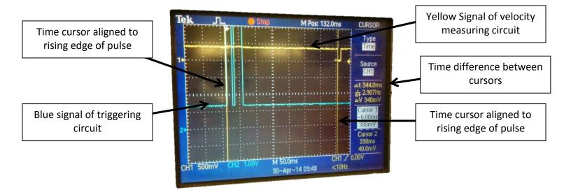
Figure 3.12: Measurement of Velocities Using Oscilloscope
