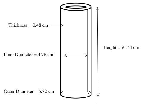
Figure 1.2: Dimensions of Tube
