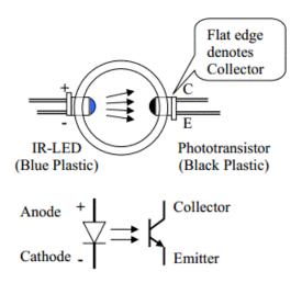
Figure 2.3: Transmitter and Receiver placement on the tube
