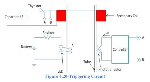
The triggering mechanism in Figure 4.20 consists of a light emitting diode (LED), a phototransistor, and a controller. When the ring travels up the ring, the light path between the LED and phototransistor is broken. When that path is broken, the controller will create a pulse. That pulse is then sent to the thyristor, thus activating the thyristor and the secondary coil. Figure 4.21 is a graph of this concept:
