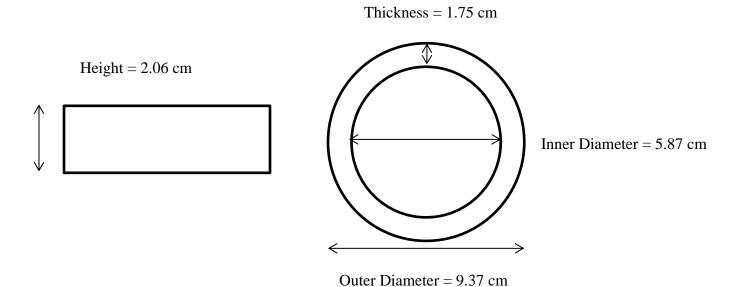
Figure 1.4: Side view and Top view of coil showing dimensions
