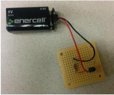
Figure 2.6: Transmitter Soldered Circuit
