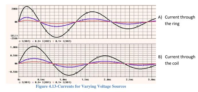
The black line represents the current with the 1000V source, the blue line represents the current with the 300V source and the red line represents the current with the 100V source. As
