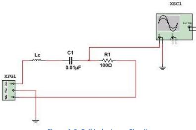
Figure 1.6: Coil Inductance Circuit
