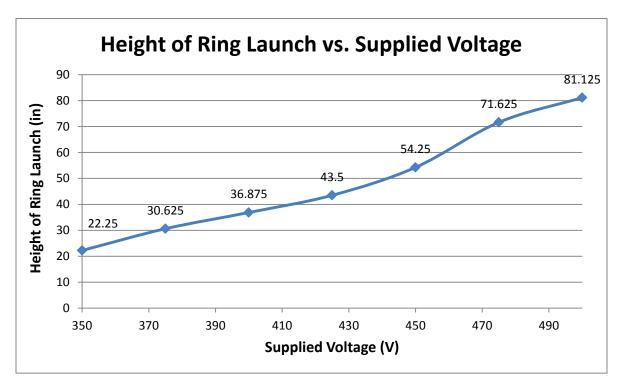
**Figure 3.7: Heights at Different Voltages**
