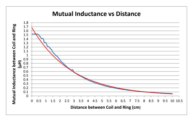
Figure 1.11: Mutual Inductance vs Distance using Lyle's Method
