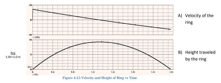
Figure 4.12A represents the velocity of the ring and Figure 4.12B represents the height traveled by the ring. Once the ring is launched, it reaches a top speed of about 14 m/s. The velocity then decreases linearly and eventually reaches 0 m/s. While the velocity is positive, that signifies when the ring is traveling upward, which can be seen in the height graph. When the
