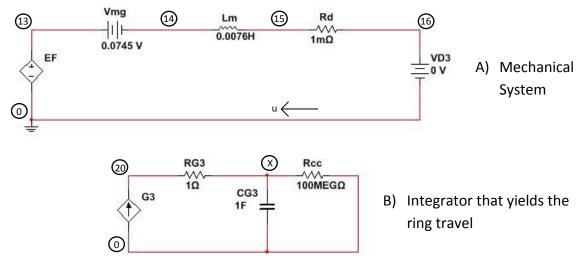
Figure 4.10-Electrical Equivalent to Mechanical System
