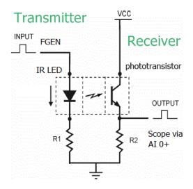
Figure 2.4: Transmitter and Receiver Circuit Configurations
