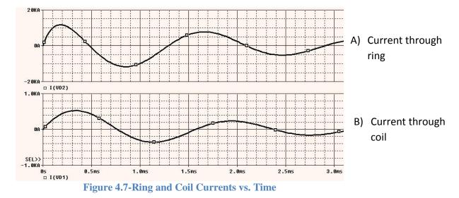
Figure 4.7A represents the current going through the ring which is around 12k amps.
