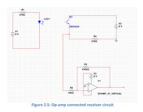
Since the transmitter and receiver circuits have to be attached directly to the sides of the tubes, portable 9V batteries were used as the voltage source, with the receiver circuit containing an extra one to power the op-amp. The actual soldered circuits are shown in figures 2.6 and 2.7. The
