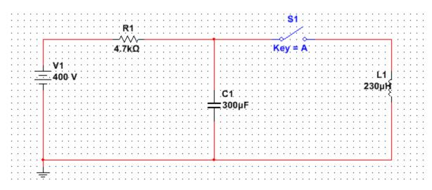
Figure 1.10: Launcher Circuit Configuration
