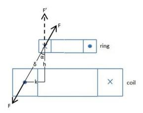
Figure 4.8-Optimizing the System (Resultant Force Calculations)
