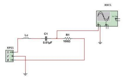
**Figure 4.5-Measuring Coil Inductance**
