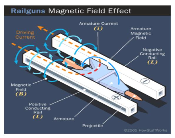
**Figure I: Railgun Structure**
