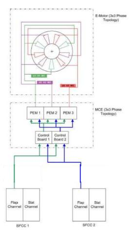
The figure above shows what a Sagem High Lift Power Drive Unit new electrical architecture could be.
