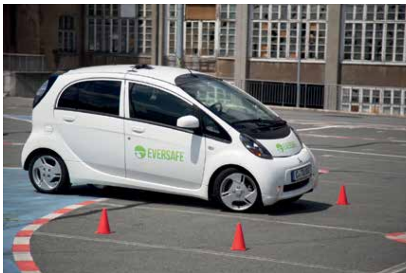
STUDYING DRIVER RESPONSE AND VEHICLE BEHAVIOUR IN CASE OF FAILURE IN ELECTRICAL POWERTRAIN.
