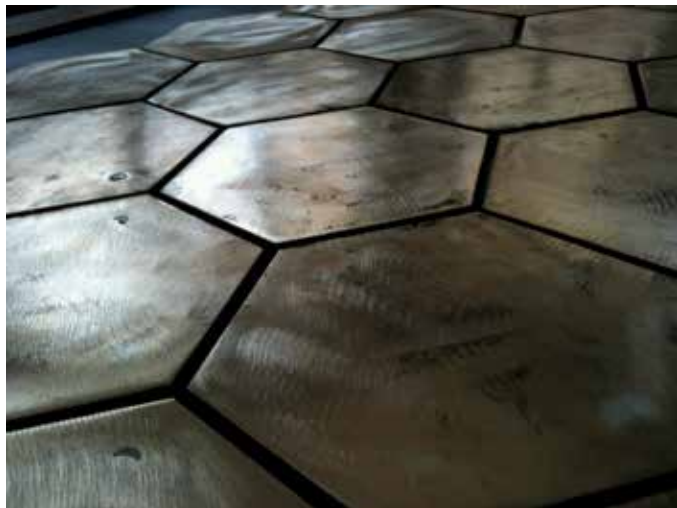
THE “POWER CARPET” (DETAIL OF HEXAGONS). THE CARPET IS PLACED ON GROUND AND IS AIMED TO ENSURE THE CONDUCTIVE ENERGY TRANSFER TO THE ULTRACAPACITOR PACK ON BOARD OF THE VEHICLE.
