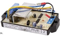
The AVR's measures the voltage between one of the alternator phases and the neutral point and adjusts the DC voltage applied to the excitation winding until reaching the desired voltage. The output stage of the device is a half-wave tyhristor output associated with a free wheeling diode.
