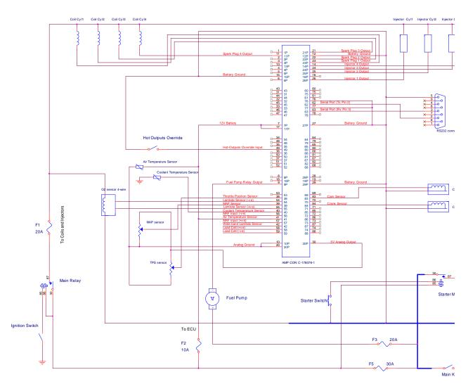
Figure 18 Basic Harness Wiring Setup
