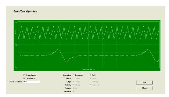
Figure 8 Oscilloscope View Dialogue
