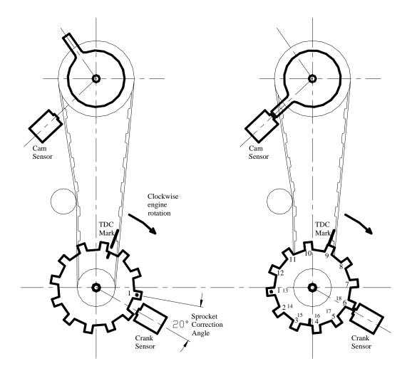
Figure 13 Case 1, Left: Determination of Sprocket Correction Angle and Tooth No 1,
