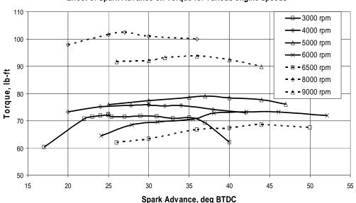
Effect of Spark Advance on Torque for various engine speeds
