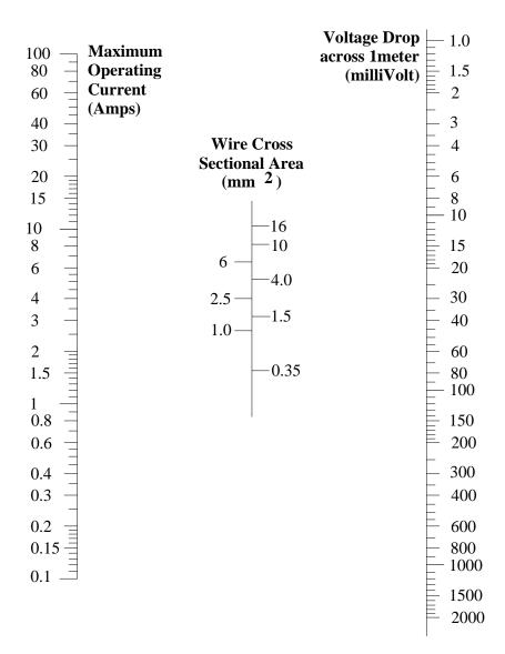
Figure 19 Wire Cross-sectional Area Namogram
