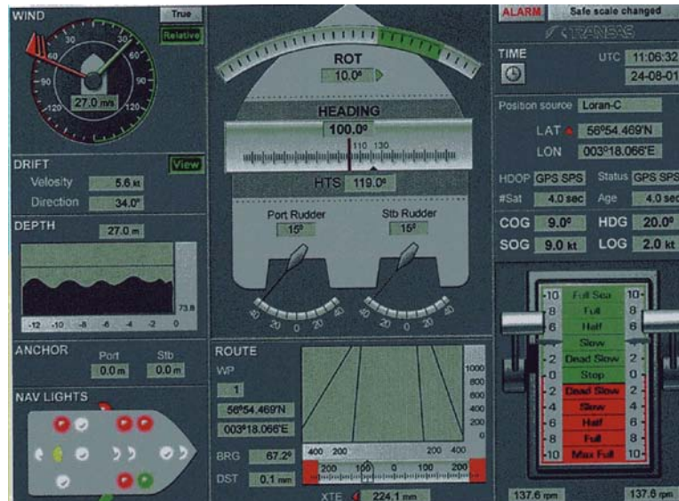
Transas Marine Flat Screen Helm Display
