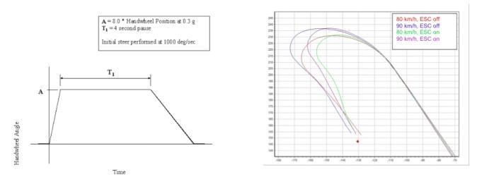
Figure 6. Steering input for J-turn test (ISO 7401) and typical vehicle path (Transport Canada)
