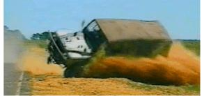
Figure 10. Example of off-road tripped rollover (credit: DV Experts)
