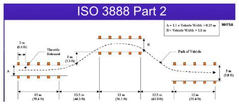
Figure 5. ISO Severe Lane Change with Obstacle Avoidance
