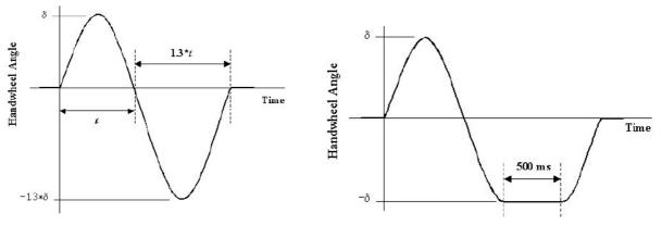
Figure 8. Steering Wheel Motion (0.7Hz Sine tests)
