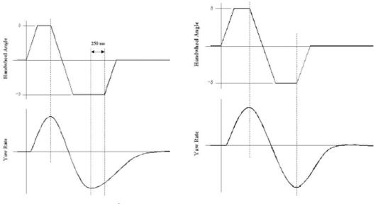
Figure 9. Steering Wheel Motion (Yaw Acceleration Tests)
