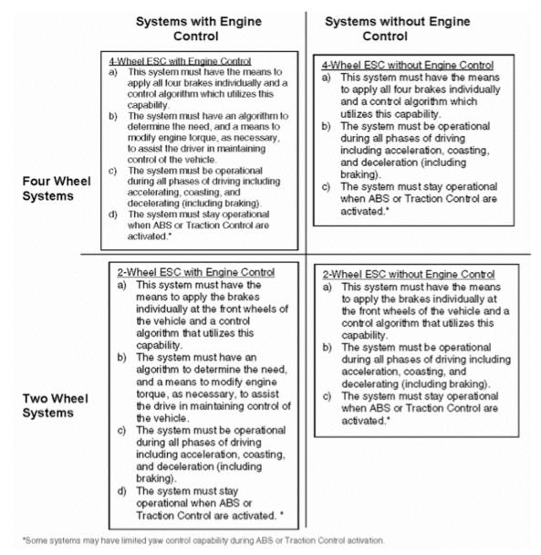
Figure 3. Extract from SAE J2564 describing the four types of ESC
