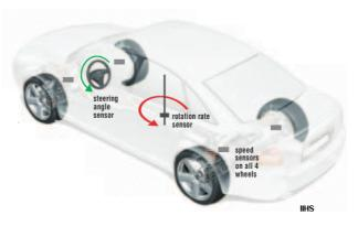
Figure 1. ESC Sensores (credit: IIHS)
