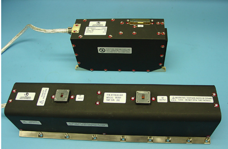
Figure 2: TWTA including high voltage power supply (top) and TWT (bottom)
