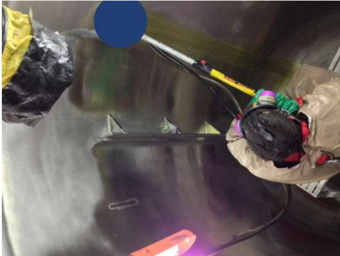
Electropolishing of vessel interior
