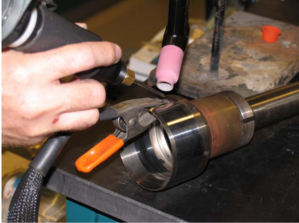
Figure 14. ESD being performed on an actual helical gear shaft containing defects at ARL.
