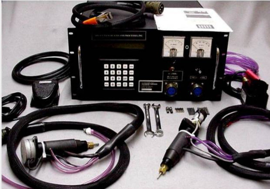
Figure 6. Equipment utilized for ESD repair of components. 1
