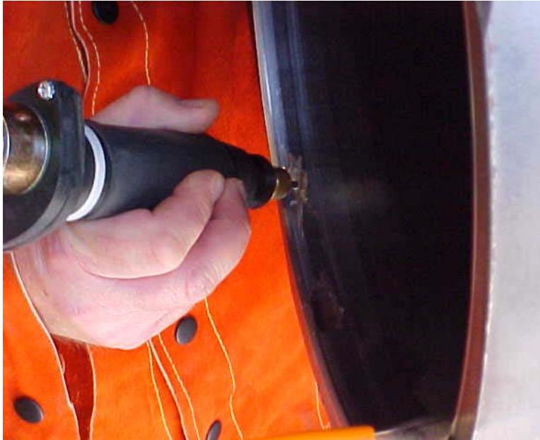
Figure 7. Photo showing ESD torch applying deposit on the inside diameter of a cradle with a rotating electrode.
