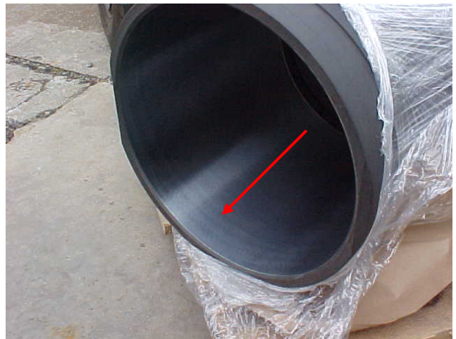
AFTER ESD REPAIR, CHROME PLATING, AND FINISH GRINDING
