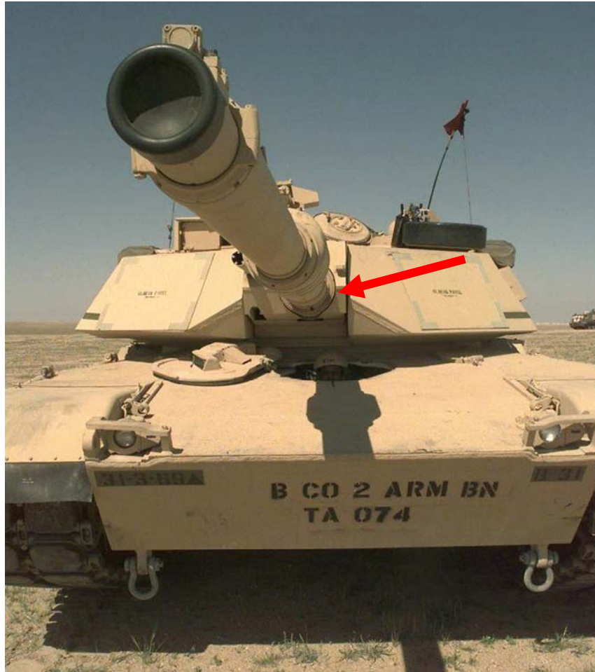
Figure 1. M1A1 main battle tank cannon cradle (arrow).
