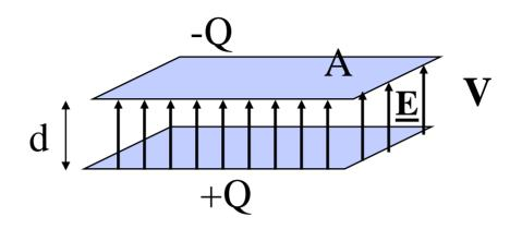
In the case of a parallel plate capacitor  $Q = \varepsilon_0 EA$  and V = Ed
