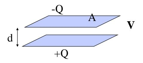
If a potential difference V is applied between the plates, charges + Q and - Q appear on the plates.
