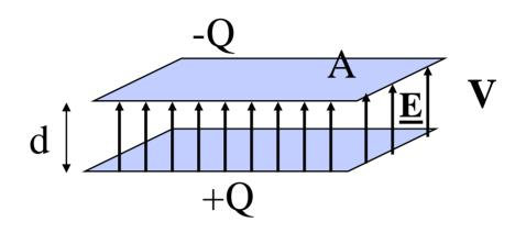
The electric potential energy can be thought of as stored in the electric field existing between the plates of the capacitor.
