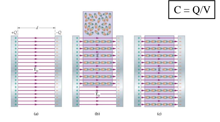
The dielectric decreases the electric field between the plates, as well as the voltage between the plates, and consequently increases the capacitance of the capacitor
