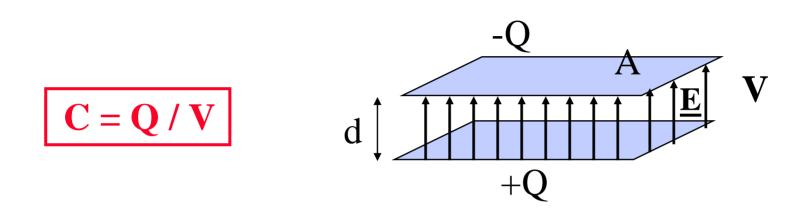
The relationship C = Q / V is valid for any charge configuration (Indeed this is the definition of capacitance or electric capacity)
