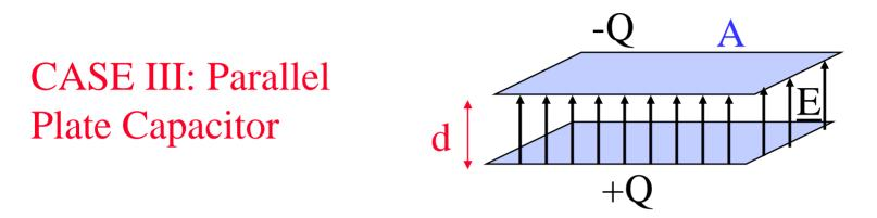
The work done in charging the plates ends up as stored potential energy of the final charge distribution
