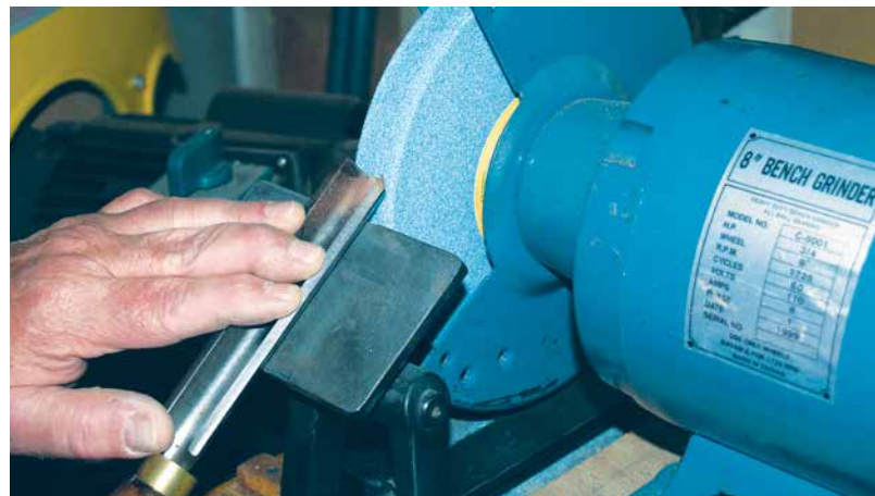
Consider learning how to hand sharpen turning tools. This allows you to place a toolrest close to the grinding wheel, eliminating many potential dangers.
