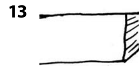
13. Side view of steep vertical edge for cutting bottom of bowl
