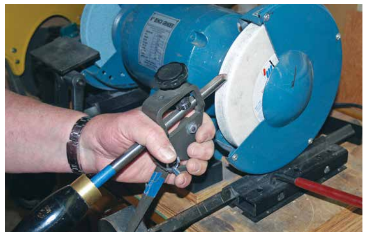
Wrong way! If the sharpening jig slips, fingers will contact the rotating wheel before the jig does.
