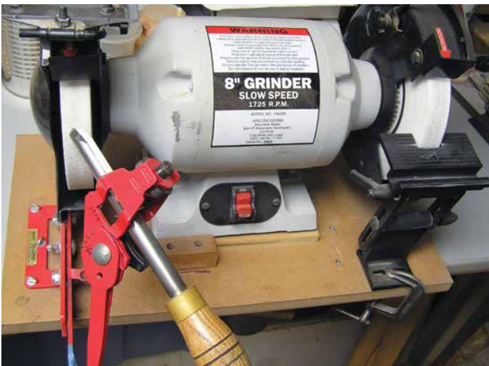
For everyday sharpening, many woodturners rely on a slow-speed grinder with two 8" × 1" white aluminum oxide wheels. On Jim Echter's machine, the left wheel has a TruGrind jig for sharpening gouges, skewers, and parting tools. The right has a Veritas adjustable-angle platform for sharpening scrapers.
