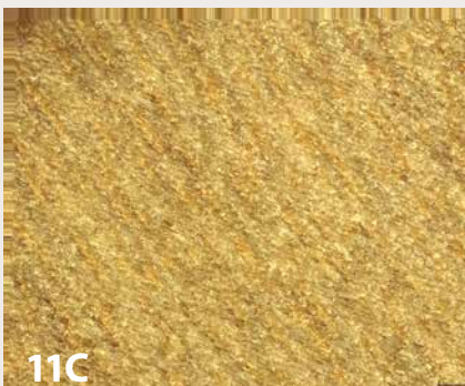
Magnification 100X, wood surfaces cut with CPM 10V gouge.
