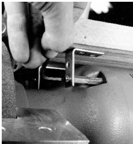
An Allen wrench tightens the shelf mounting bracket. Allen head works well in tight space.
