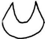
15. Thin skew-like edge can cause vibration 16. Additional mass behind edge reduces vibration
