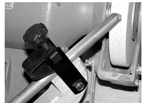
A jig may be helpful in some situations of learning to grind.
