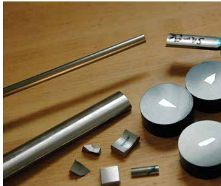
Sections of lathe tools embedded in composite materials and prepared for emission (spark) test.
