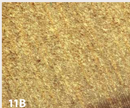
Magnification 100X, wood surfaces cut with PM 2060 gouge.
