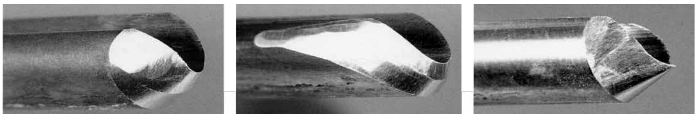
3. Three different grinds: A mild side grind on a Glaser gouge, left. Center, a more pronounced side grind on a Sorby deep bowl gouge. And right, a nib-gouge grind.
