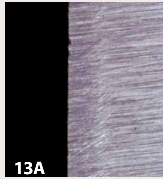
13A Cutting edge of a M2 HSS skew, ground and honed (200X).
