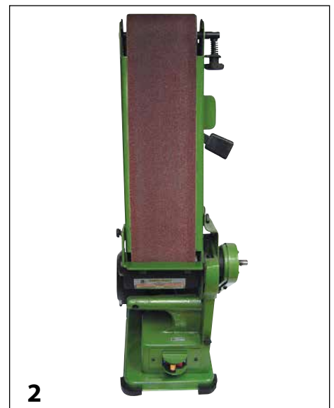
2 For this modification, unpack the parts but do not mount the disk sander or its table. Also, remove the back cover and bottom dust port, the sanding-belt guard, and the drive-belt cover.
