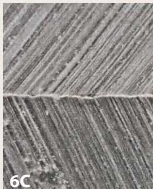
Edge view of skew chisel edge, ground (200X).
