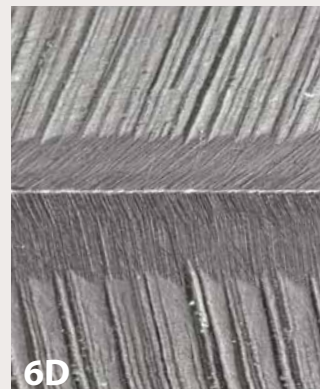
Edge view of skew chisel, ground and honed (200X).
