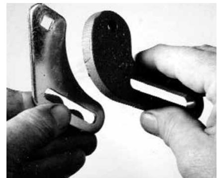
Cast iron tool rest holder is much heavier than the stamped steel ones originally on the author's grinder.
