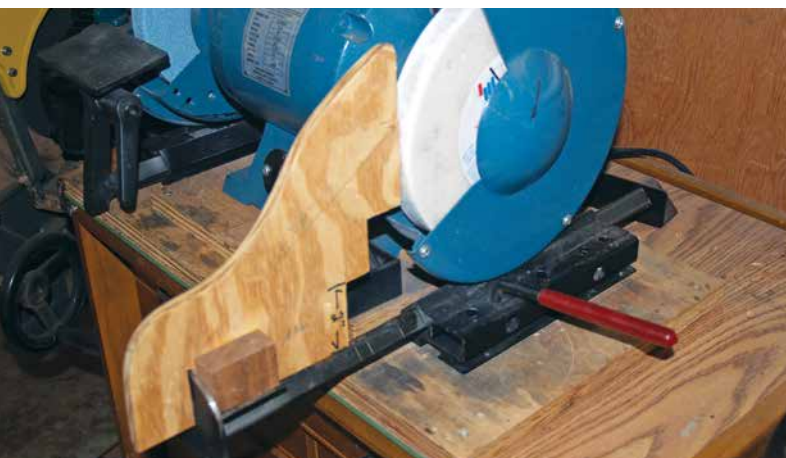
Using a simple shopmade template to set up your sharpening jig for repeatable distances saves time and tool wear.
