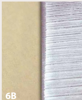
Skew chisel edge, ground and honed (20X).
