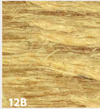
12B Resulting cut wood surface (100X).
