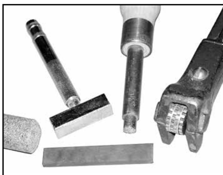
Wheel dresser examples left to right: gray dressing stick, tee diamond, round diamond, star-wheel. In the foreground is a boron carbide stick.
