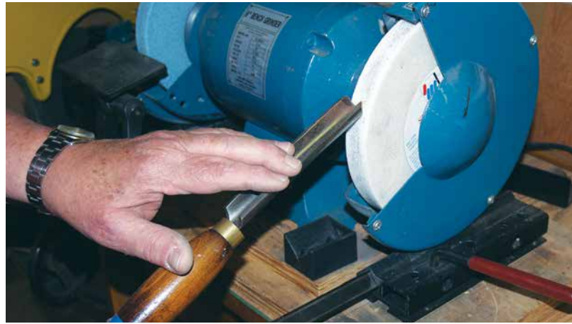
Potential danger: Using a long fixture arm and a blunt sharpening angle brings the tip of the tool too close to the wheel's equator. If the arm of the jig slips or too much pressure is exerted, it could cause the tool to jam against the wheel.
