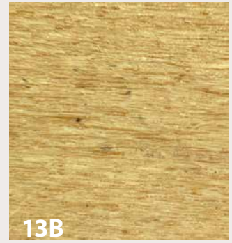
13B Resulting cut wood surface (100X).
