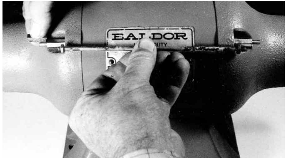
The author holds the old motor bolt in front of the mounting bracket, which already has all-thread and one coupling nut installed. The second coupler is needed to install the angle bracket.
