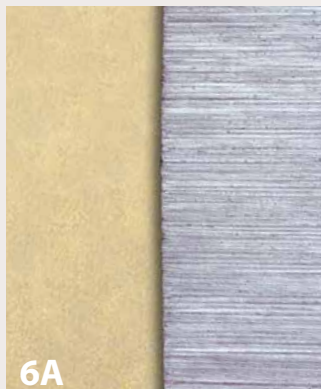
Skew chisel edge, bevel ground only (20X).
