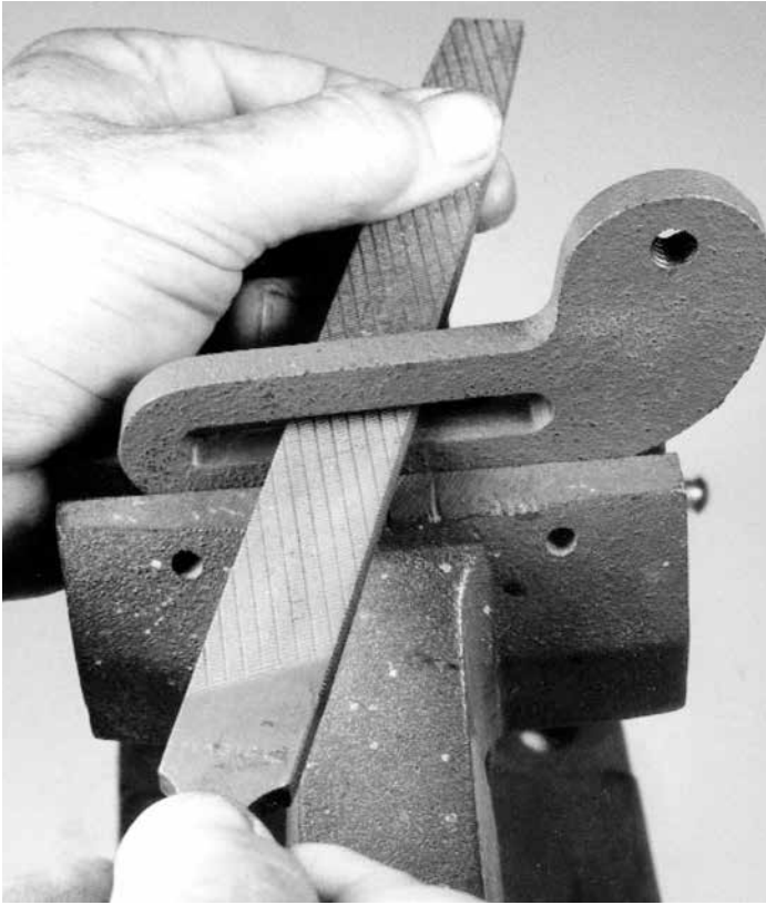
A file is used to open up the adjusting slot in the tool rest support. Also shown is the newly enlarged and threaded hole for the tool rest.
