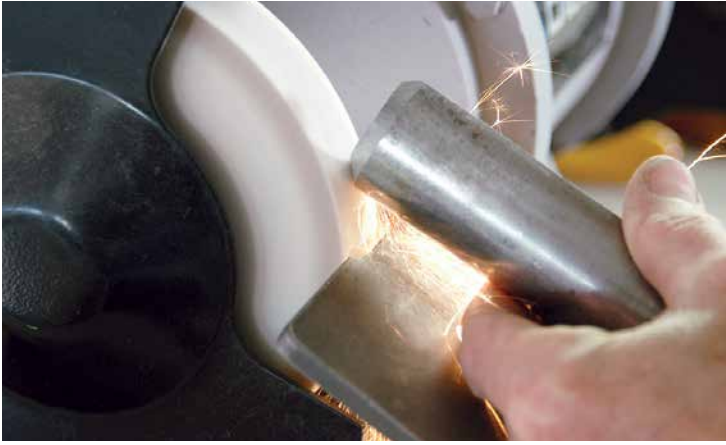
As a general guideline, high-carbon steel sparks remind some turners of sparklers. At the grinder, you should notice a complex shower of sparks.
