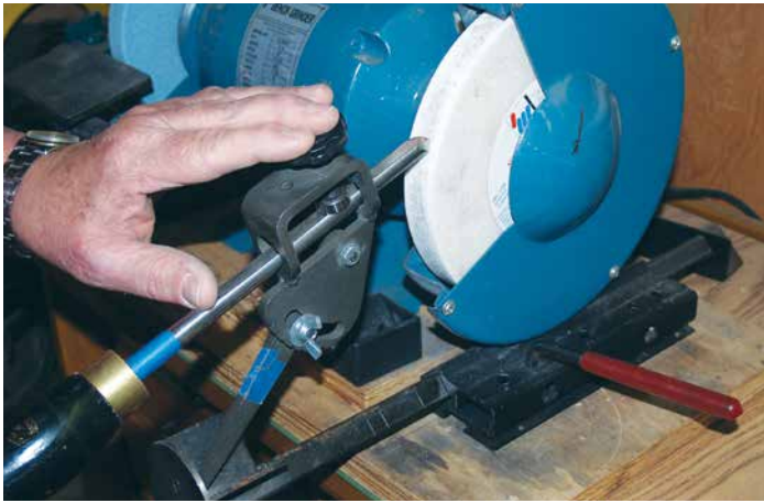
A safer way to hold the jig is on the top. If a slip occurs, the hand is protected.
