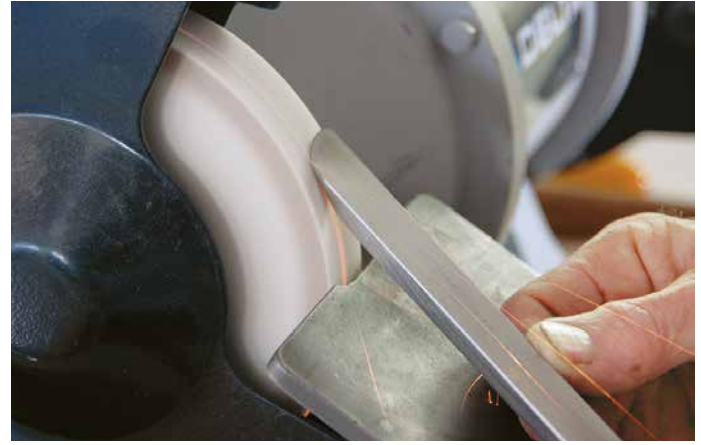
As a general guideline, high-speed steel (HSS) sparks remind some turners of tracer bullets and tend to be individual sparks. Note: This test is not always conclusive for HSS.
