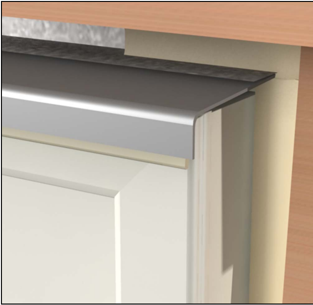
Figure 23 Apply sealant between window and exterior finish.
