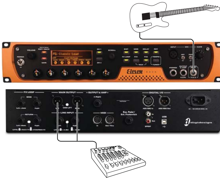
Figure 5. Eleven Rack connected directly to the PA mixer
