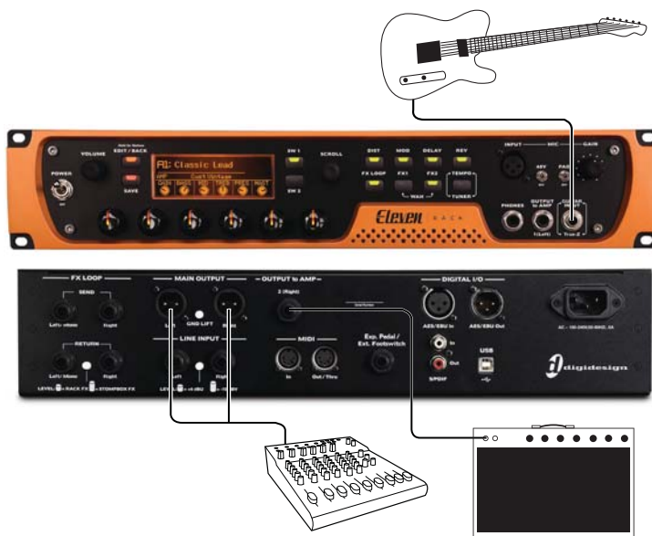
Figure 6. Eleven Rack connected to the PA mixer and an onstage amplifier
