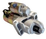
Most late model boats reverse the prop shaft rotation in the transmission AND NOT in the engine. Because of this, use API Marine starter #10095 or #10099 on late GM blocks using a 14" flywheel with "reverse rotation."
