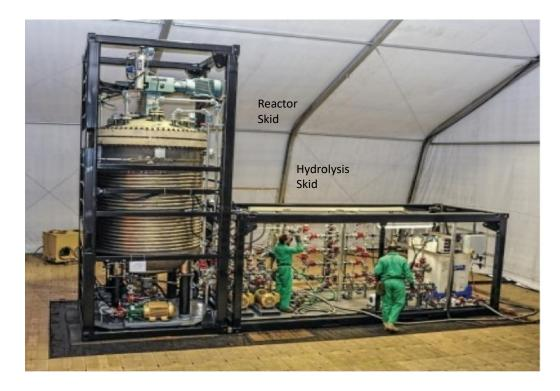
**Figure 3.** Army Field Deployable Hydrolysis System – Reactor and Hydrolysis Sections (courtesy of the U.S. Army)
