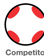
Figure 11. Magnetic bead aggregation comparison. Drawing of one well of a 96-well plate from the top view. Red bar and circles depict where the magnets are located when placing the 96-well plate on the handheld magnet.
