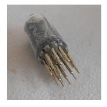
Insert the tube with sockets into the PCB from the side with the pre-soldered ICs. Push firmly in. You may need to wiggle a little from side to side, to get all the sockets to fully go into the holes, to the level as shown below.
