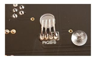
To prevent excess stray light, you can add small pieces of the 5mm heat shrink over the LEDs. It is not necessary to shrink the tubing. If you choose to shrink it, be careful as it may shrink so narrow that almost no light comes out.
