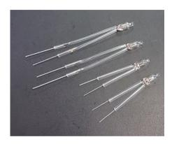
Finally, solder the neons in place on the PCB, with the taller neons at the back. The glass cover tubes can be placed over later.
