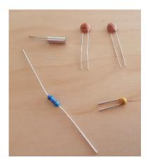
The 10pF capacitor is usually marked '10' and not surprisingly the 33pF is marked '33'. The 100nF is marked 104. Don't switch C5 and C6 or the timekeeping will be very slow.
