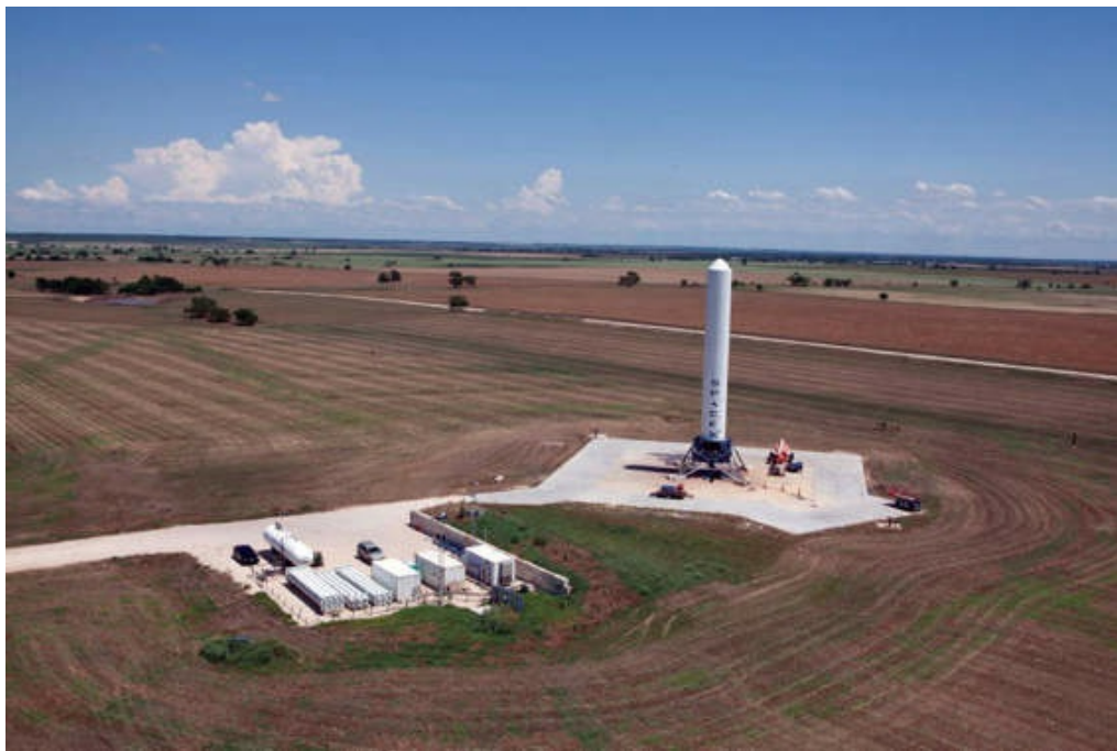
SpaceX tests new engines and crafts at a site in McGregor, Texas. Here the company is testing a reusable rocket, code-named “Grasshopper,” that can land itself. Photograph courtesy of SpaceX
