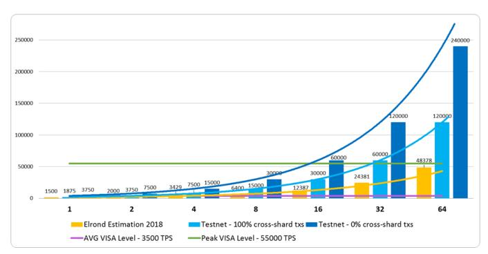
Fig. 12: Network throughput measured in transactions per seconds with a global network speed of 8 MB/s
