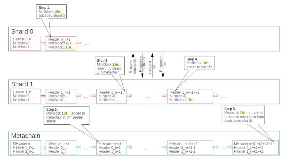
Fig. 4: Cross-shard transaction processing
