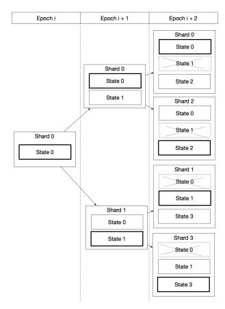
Fig. 3: Shard redundancy across epochs
