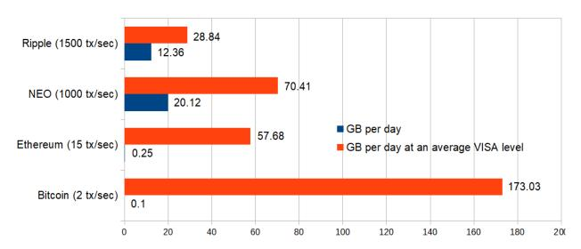
Fig. 11: Storage Estimation - Validated distributed architectures working at an average of VISA TPS
