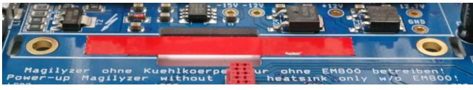
Flip the PCB and solder the voltage regulator exact in the middle of the cutout.
