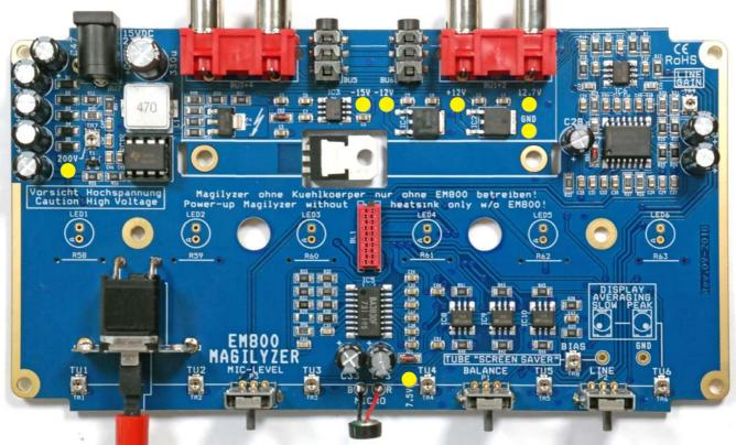
When everything is ok, turn off the Analyzer and **fit after a short waiting period the NE555 (IC12)** into its socket. Turn on again the Analyzer.
