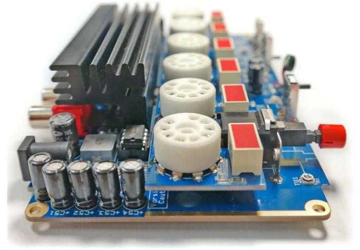
Now you can start the first test run with fitted EM800 tubes and the built-in microphone. But be aware as the high voltage is not touch-protected yet.
