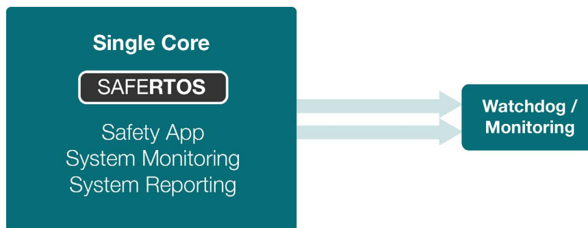
Figure 4-1 Single Processor Architecture
