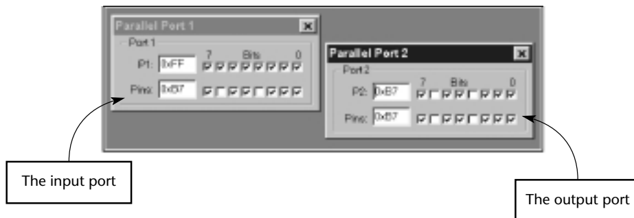
FIGURE 4.3 The output from the program in Listing 4.1 produced using the Keil hardware simulator included on the CD. Note the difference between the Port 1 latch value (0xFF) and the pin value (0xB7)
