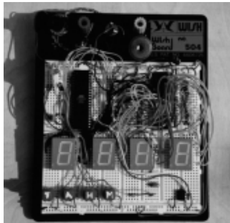
FIGURE 1.7 An example of a simple 8051-based alarm clock assembled on a breadboard. The board was assembled by Neeraj Kachhwaha, Bresley Lim, Melvin Lim and Henry Tam. Photograph by Michael Pont
