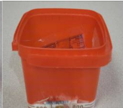
Figure 3-3: The containers resulting from the preliminary tests. A) Container that failed to fill completely along the top edge (the alien tag is around the corner on the lower right hand side). B) Another container with similar aspects and if you closely at the tag, it is almost completely separated from the sidewall. C) The IML film on this container slipped due to the addition of the tag and the tag is also not attached.
