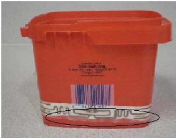
Figure 3-3: The containers resulting from the preliminary tests. A) Container that failed to fill completely along the top edge (the alien tag is around the corner on the lower right hand side). B) Another container with similar aspects and if you closely at the tag, it is almost completely separated from the sidewall. C) The IML film on this container slipped due to the addition of the tag and the tag is also not attached.
