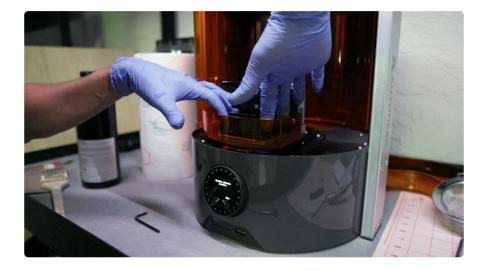
From here we can loosen the build head - let it drop down and push on all four corners to lay it flat. Once its all straight and level, we can tighten it back up and complete the process.
