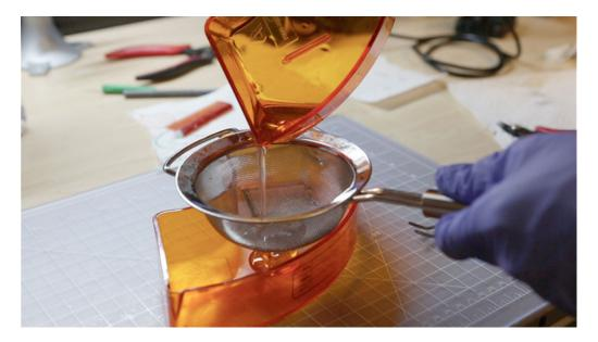
If theres a lot of bits and pieces, use a fine mesh strainer to quickly filter out smaller debris into the second tray. The build head is easy to clean after each print, just wipe off any remains.
