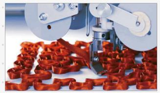
Taping and cording with W-head
