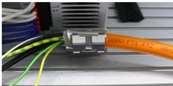
Fig. 3-5: Shielded three-phase cable with PE conductor
