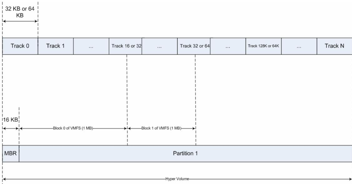
Figure 10 Pictorial representation: Hypervolume to Symmetrix track mapping
