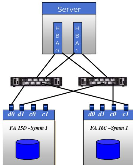
Figure 8 One host, two switches, and one Symmetrix array
