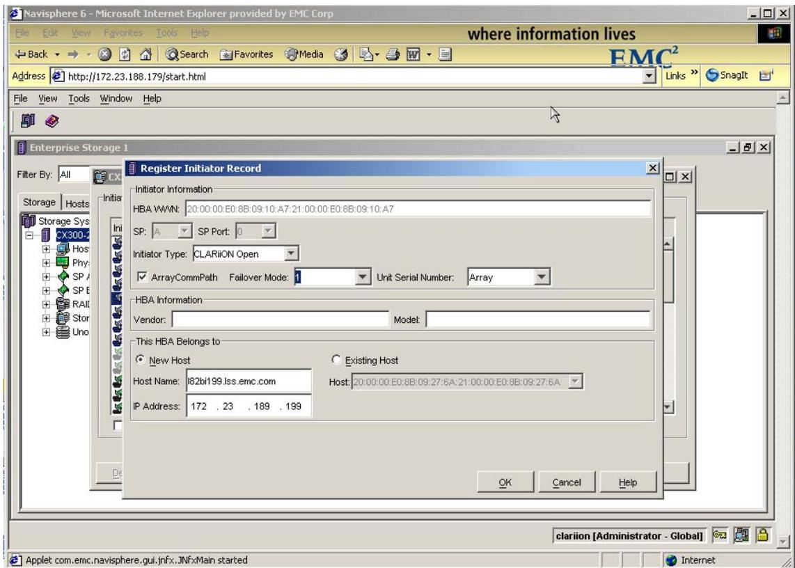
Figure 22 Registering for a failover-enabled environment example
