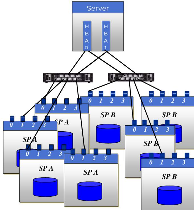
Figure 19 One host, two switches, and four CLARiiON arrays
