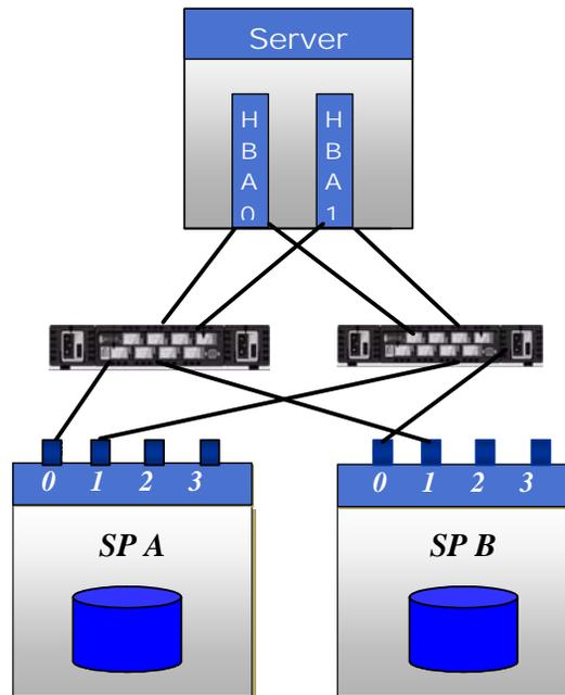
Figure 18 One host, two switches, and one CLARiiON array
