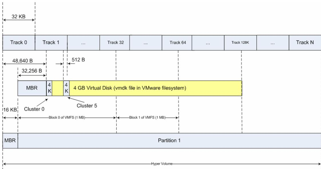
Figure 11 Track misalignment: VMware ESX Servers using VMware file system
