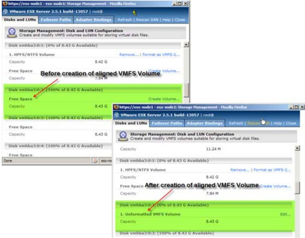
Figure 16 View of aligned partitions in the MUI
