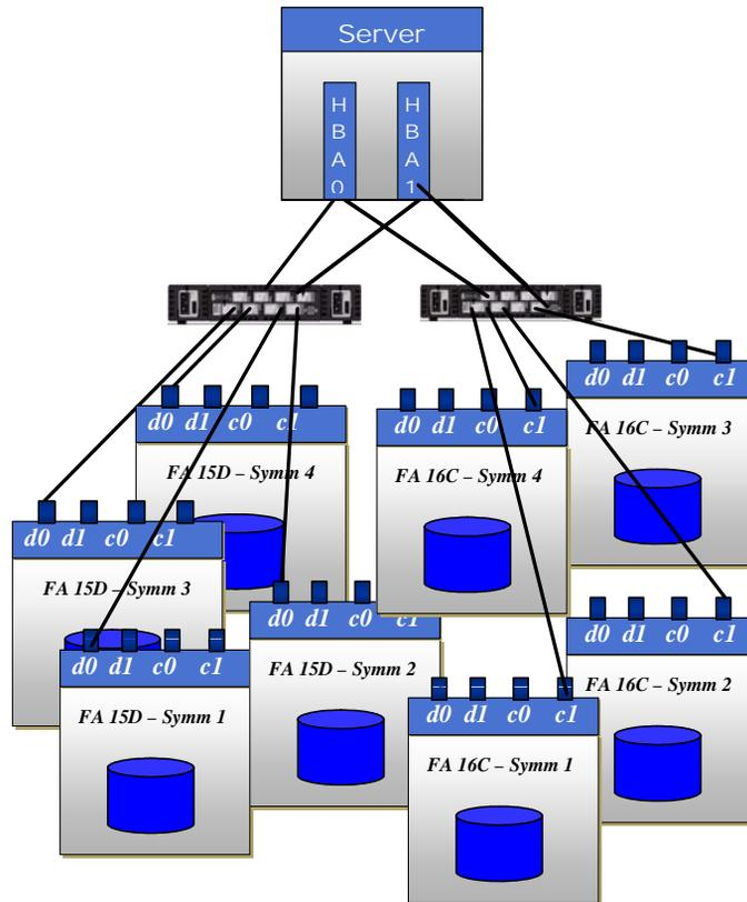
Figure 9 One host, two switches, and four Symmetrix arrays
