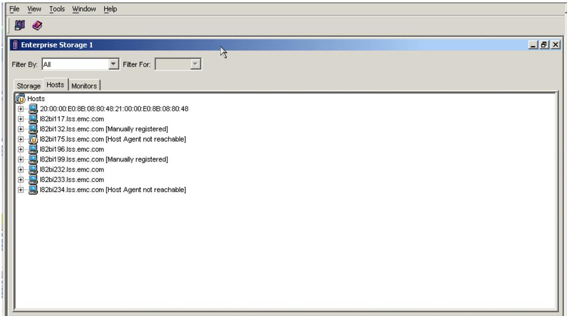
Figure 24 Host reported as attached, but manually registered example
