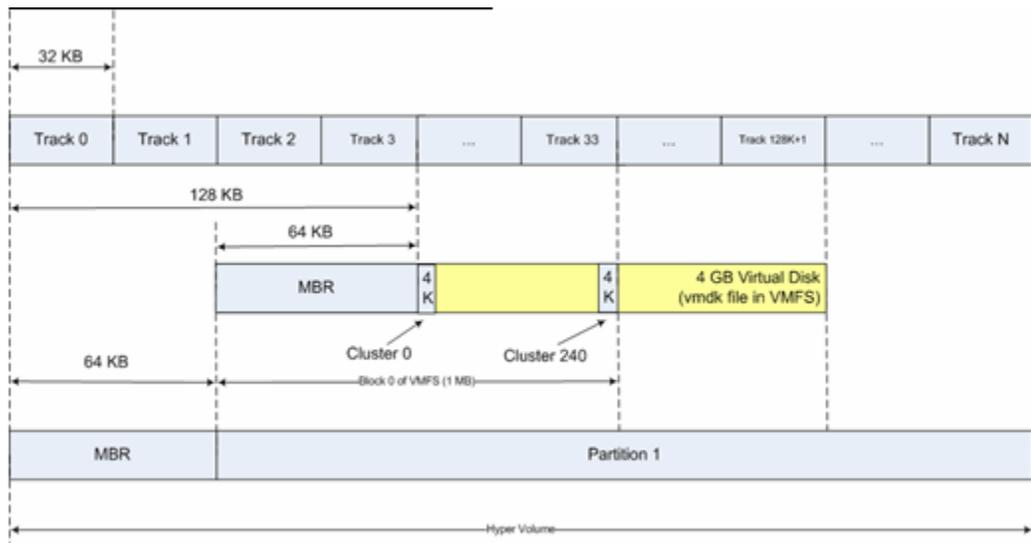
Figure 17 Track aligned VMware file system and virtual disks
