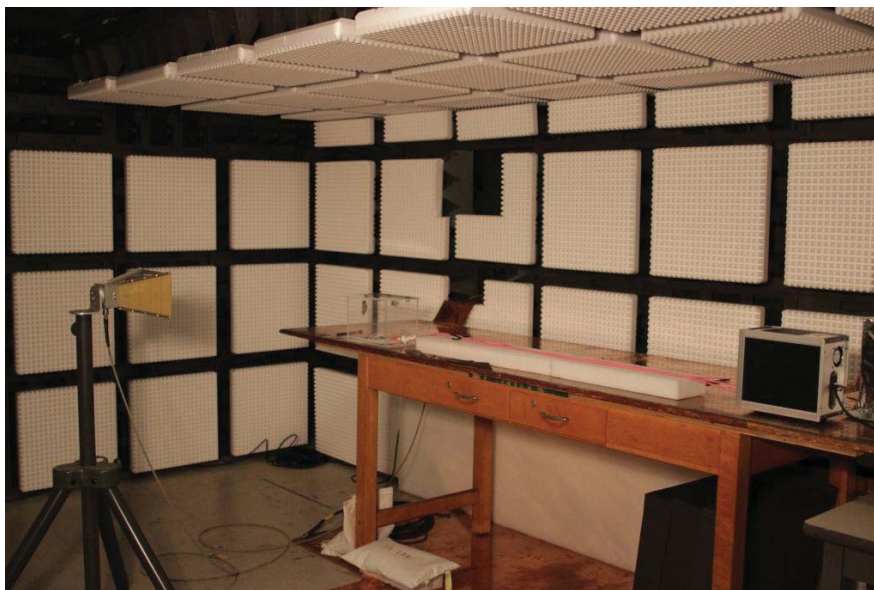
Figure D.3-10: RE02 Typical Antenna Setup, Above 1 GHz
