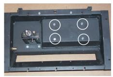
**14)** Remove the 4 Phillips head screws from the sides of the valve bracket and remove valve.
