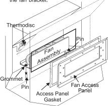
Lift fan off of the 2 pins, tip forward and pull through the firebox opening.
