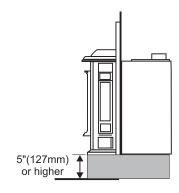
When the Insert is installed in a fireplace that is elevated 5" or higher, no floor protection is required in front of the appliance.
