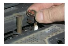
Unscrew the pilot orifice with the allen key and replace with the LP pilot orifice in the kit.
