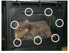
Remove the 7 nuts holding the Front Glass Bracket to the front face. CAUTION: Don't let the glass drop.
