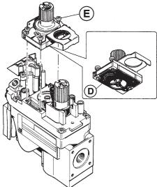
8) Pull off the pilot cap to expose the pilot orifice.
