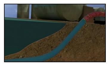
First plug is deployed from one end of the pipeline toward the defect.
