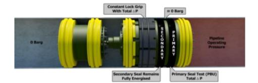
Figure 15: Primary Seal Test
