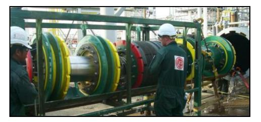
Figure 12: 36" Remote Tecno Plug™ Deployment Malaysia
