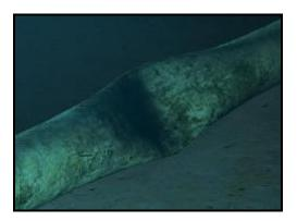
Figure 1: Unpiggable Defect in Pipeline
