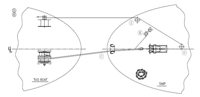
6. Lash the towing with the stopper rope so that towing rope won't drop loose.
