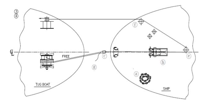
4. Reel the messenger rope on to the warping end of the vessel's mooring winch by way of the pedestal roller and the fairlead roller .
