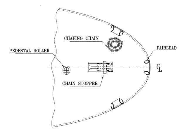
The forward Emergency Towing System consists of the following equipment.
