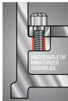
**Inaccessible or Miniaturized Assemblies.** Heli-Coil Screw-Lock inserts permit the installation of the lock from the front or top. No blind fumbling for assembly of lock washers or lock nuts behind or underneath.
