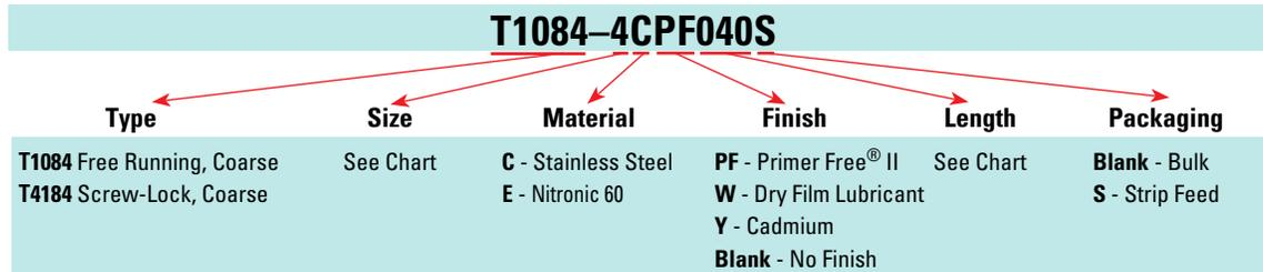
**Complete Part No. Example:** Free Running Insert; M4 x 0.7; Tap Stainless Steel; Primer Free II; 1 dia.; On Strip
