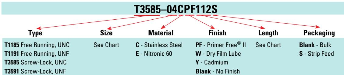
**Complete Part No. Example:** Screw-locking Insert; #4-40; Stainless Steel; Primer Free II, 1 dia.; On Strip
