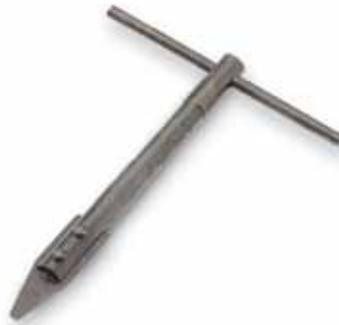
Strike the head of the tool with a light blow. Maintaining a steady pressure of blade against insert, turn the extracting tool counterclockwise until the insert is removed.
