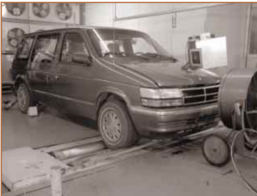
Emissions test on an aftermarket conversion being performed on the Colorado Department of Health and Environment's chassis dynamometer
