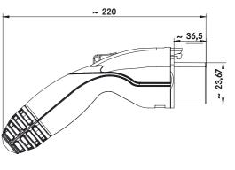
The LAPP CHARGE vehicle plug type GB is a connector for charging electric vehicles that establishes the connection between the charging cable set and the vehicle's vehicle socket.
