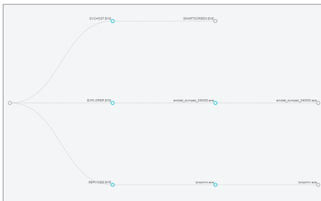
Figure 43 – Bromium Controller process interaction graph of emotet_dumped_240000.exe. It launches itself and creates service a called “ipropmini”, which closely matches the behavior shown by 15.exe.
