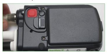
Disconnect the drive-line from the original controller by pressing down on the red tab and gently pulling on the metal end. The pump will stop and an alarm will sound. Note: The alarm will continue until the original controller is put to sleep. You can silence the alarm by pressing the silence button. Getting the replacement controller connected and pump restarted is the first priority.
