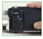
Connect the replacement Controller by aligning the BLACK ARROWS on the driveline and replacement Controller and gently pushing the driveline into the replacement Controller. The pump should restart, if not complete the following steps:
